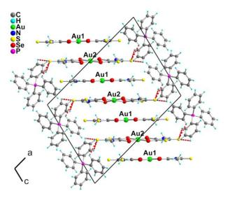
**Figure 3.** Projection view of the unit cell of  $[Ph_4P][Au(Me-thiazds)_2]_2$  along b. C $-H^{\bullet\bullet\bullet}S$  interactions shorter than 3.1 Å are highlighted as dashed red lines.
