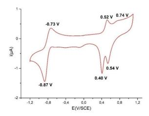
**Figure 2.** Cyclic voltammogram of [Et<sub>4</sub>N][Au(Me-thiazds)<sub>2</sub>] recorded in CH<sub>2</sub>Cl<sub>2</sub>-Bu<sub>4</sub>NPF<sub>6</sub> 0.1 M at a platinum electrode, scan rate 100 mVs<sup>-1</sup>.
