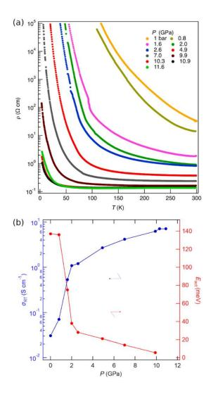
**Figure 6.** (a)Temperature dependence of the resistivity of [PPh<sub>4</sub>][Au(Me-thiazds)<sub>2</sub>]<sub>2</sub> at different pressures, (b) Pressure dependence of room temperature conductivity and activation energy
