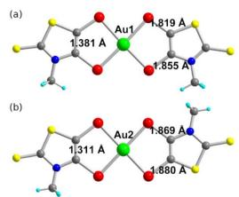
**Figure 4.** Details of both crystallographically independent gold complexes (*cis*-Au1, *trans*-Au2) in [Ph<sub>4</sub>P][Au(Me-thiazds)<sub>2</sub>]<sub>2</sub>, with selected intramolecular bond distances.
