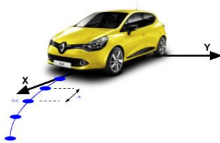
Fig. 1. Car motion trajectory definition in the car coordinates system.
