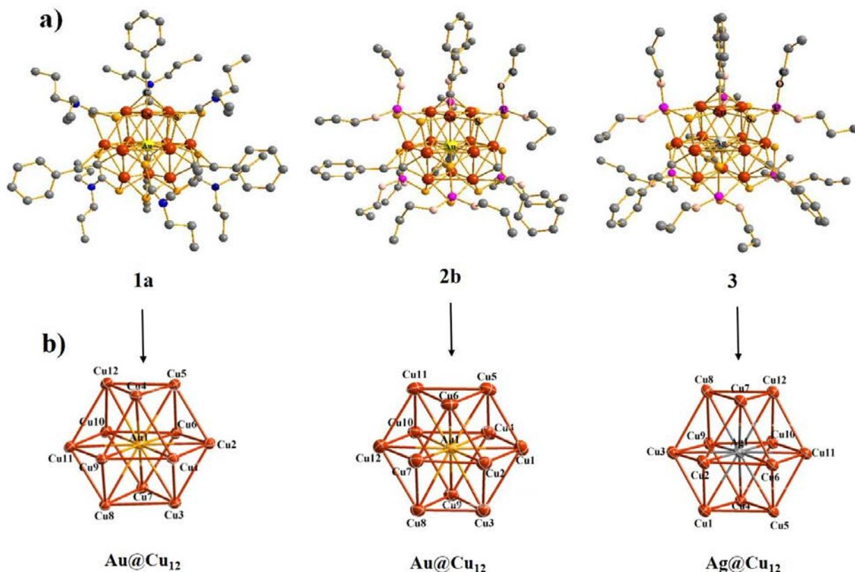
**Figure 1.** (a) Single crystal X-ray structures of cluster cations **1a**<sup>+</sup>, **2b**<sup>+</sup>, and **3**<sup>+</sup> with hydrogen atoms omitted for clarity; (b) Thermal ellipsoid drawings (50% probability) of centered cuboctahedral kernels M@Cu<sub>12</sub> (M = Au, Ag).
