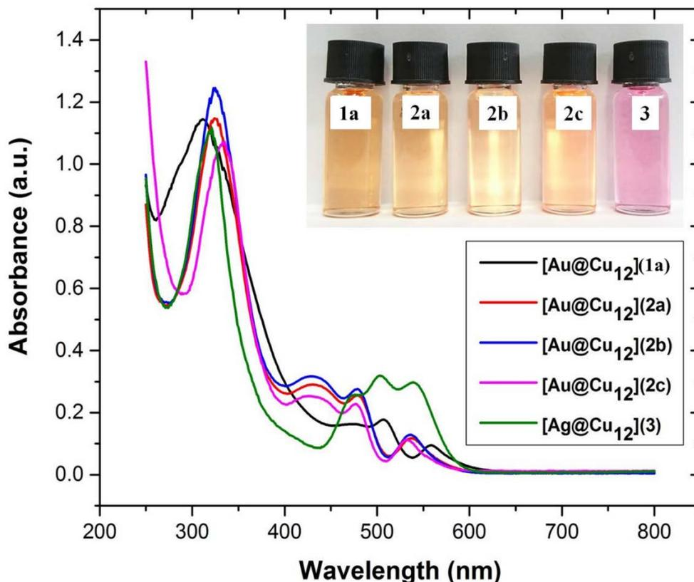
**Figure 2.** UV-vis absorption spectra of salts of **1a<sup>+</sup>**, **2a<sup>+</sup>**, **2b<sup>+</sup>**, **2c<sup>+</sup>**, and **3<sup>+</sup>** in CH<sub>2</sub>Cl<sub>2</sub>. The inset shows photographs in CH<sub>2</sub>Cl<sub>2</sub> at ambient temperature.
