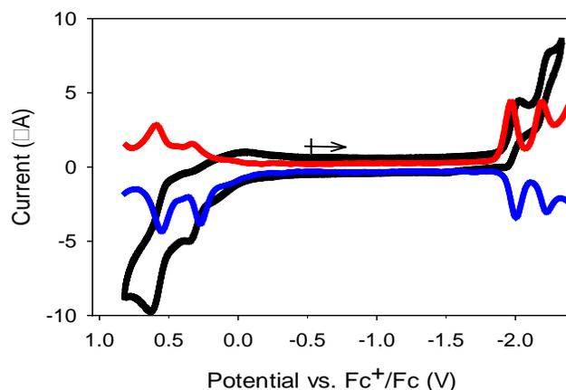
**Figure 4.** Cyclic voltammogram (black) and differential pulse voltammograms (blue and red line) of  $2a^+$  (0.6 mM) at 233 K in  $CH_2Cl_2$  containing 0.1 M  $[tBu_4N][B(C_6F_5)_4]$  solution under  $N_2$  atmosphere.
