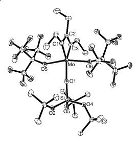
**Figure 3.** ORTEP diagram of **MoSiF9-MCBD** with thermal displacement parameters drawn at 30% probability; hydrogen atoms are omitted for clarity. Selected bond lengths [Å] and angles [°]: Mo-C1 1.877(5), Mo-C3 1.924(6), Mo-O1 1.869(4), Mo-O5 2.058(3), Mo-O6 2.053(3), C1-C2 1.480(8), C2-C3 1.424(8), Mo-O1-Si 173.3(2), O1-Mo-C1 131.9(2), O1-Mo-C3 144.8(2), O5-Mo-O6 162.56(14).
