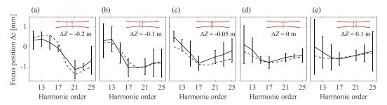
FIGURE 5: Measured (solid line) and simulated (dashed line) focus positions of harmonics 11-25 for five different generation positions in relation to the IR focus. The insets indicate the geometry of the generation in the five cases. The medium is represented by the vertical blue line, while the position of the IR focus is indicated in red. The error bars are obtained from the standard deviation of the fit performed in Figure 3.
