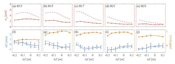
Figure 6: Simulated (dashed red) and measured waist size (solid red) as a function of generation position, for harmonic 13, 15, 17, 21, and 23 (a–e). Measured (solid blue) and simulated (dashed blue) focus positions, and measured yield (orange) as a function of generation position for the same harmonic orders (f–j).
