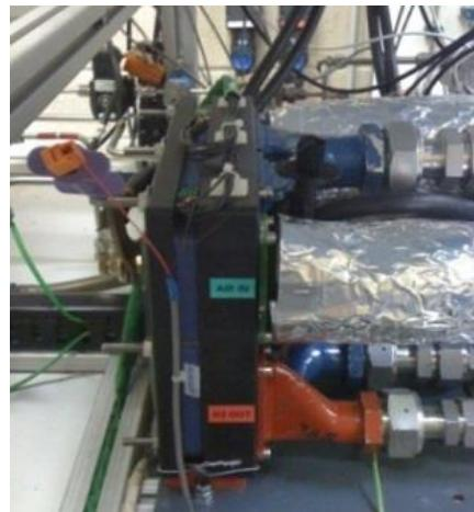
*The experimented 8 cell PEMFC (operated with pure H<sub>2</sub>)*
