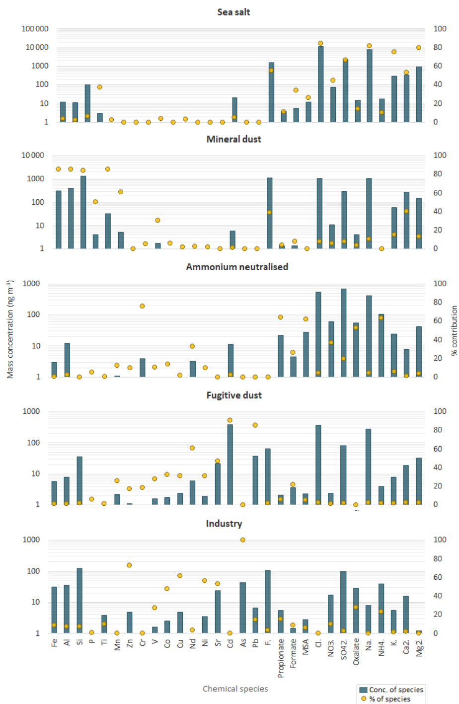
Figure 6. Profiles of the five components identified by the PMF analysis. Blue bars denote the mass concentrations of individual elements/ionic species (left logarithmic axis, \text{ng m}^{-3} ), while the yellow points indicate the percent of species attributed to the source (right axis).
