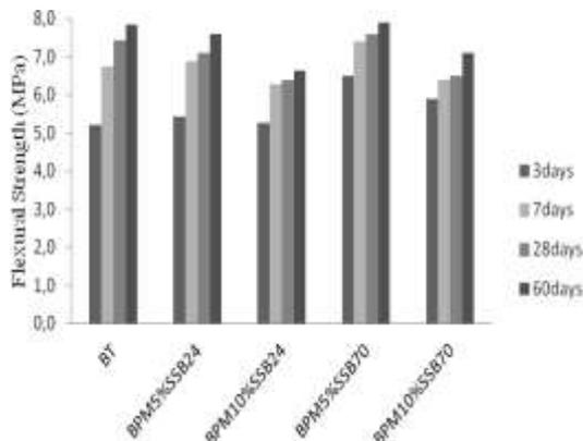
Figure 7. Evolution of the flexural strength of different types of concrete
