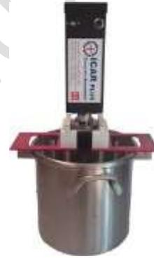
**Figure 2.** The ICAR Rheometer
