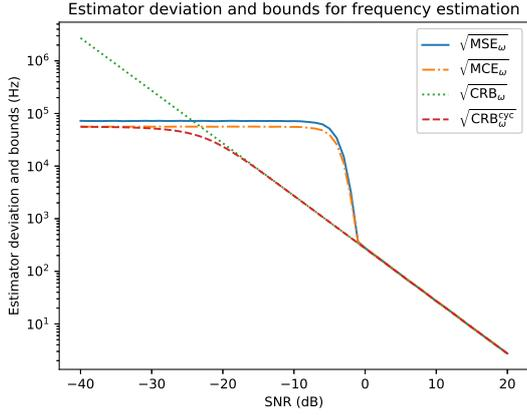
Figure 5: Estimator deviation and bounds for frequency estimation.
