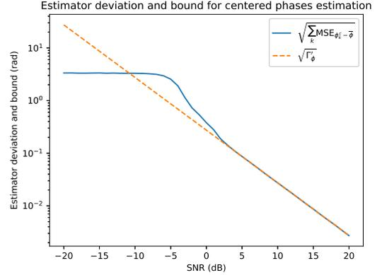
Figure 7: Deviation of the estimates of  $\phi^c$  and corresponding bound  $\sqrt{\Gamma'_\phi}$ .
