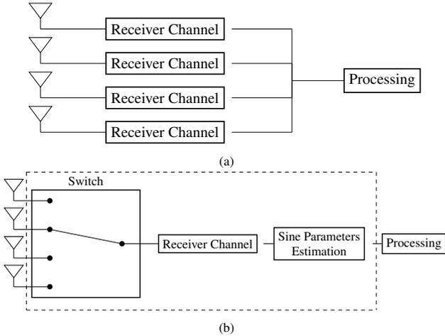
Figure 1: Examples of two systems for sampling and processing the signals received by an array of antenna. On the left is the most classical system, associating a receiver channel to each antenna. On the right is the subject of this paper, where all antennas are sampled by a single receiver channel through a switch.
