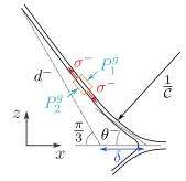
FIGURE 7. Schematic of the pushed film with the normal forces applied.
