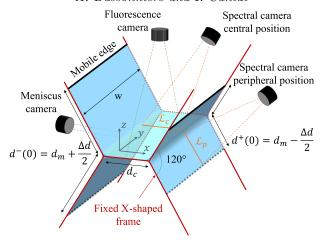
FIGURE 1. Schematic of the experimental setup showing the mechanical device controlling film deformation and the different optical devices used to monitor the film motion.
