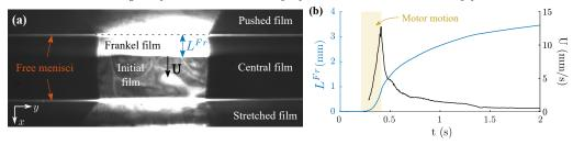
FIGURE 3. (a) Image of the fluorescence camera (top view) after the deformation showing the Frankel film extraction. This Frankel film is invariant in the y direction and the black parts on both sides are due to the fact that the illuminated domain size is smaller than W. (b) Typical Frankel film length  $L^{Fr}$  (blue) and velocity  $U = dL^{Fr}/dt$  (black) evolution with time for  $\Delta d = 10$  mm, V = 50 mm/s and  $d_m = 12$  mm. Yellow shaded area indicates when the motors move.
