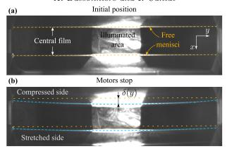
FIGURE 5. (a) Fluorescence image of the central film at the initial state showing the position of the free menisci (yellow dashed line). (b) Fluorescence image at the end of the motor motion. New positions of the menisci are highlighted by dashed blue lines.
