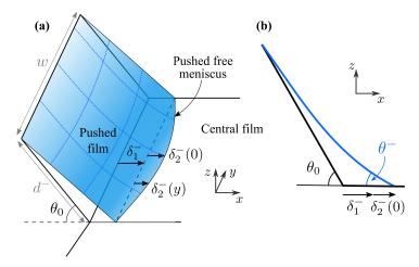
FIGURE 8. (a) 3D schematic of the pushed film shape ensuring zero mean curvature. (b)
