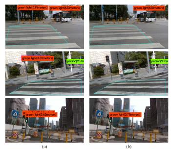
Fig. 10. The detected results by YOLOv4 (a) and our method (b).
