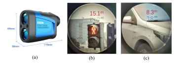
Fig. 11. The laser rangefinder and its use cases. The distances labeled in red are the results measured by our system and the distances marked in dark blue are that measured by the rangefinder which represent the ground truth. (a) The laser rangefinder; (b) The measurement case of PTL; (c) The measurement case of vehicle.
