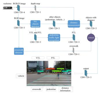
Fig. 3. The crosswalk scene understanding system. The crosswalk, pedestrian, vehicle and PTL are detected. The distance of key objects(pedestrian, vehicle, PTL...) are measured. VTL:vehicle traffic light; PTL:pedestrian traffic light.
