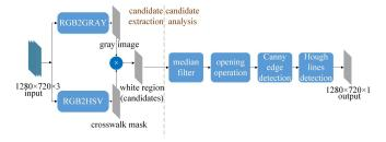
Fig. 4. The framework of crosswalk detector.
