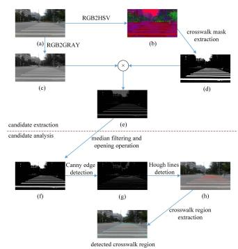
Fig. 5. Diagram of candidate extraction and candidate analysis: (a) input image; (b) HSV image; (c) gray image; (d) crosswalk mask; (e) white region(candidates); (f) result of median filter; (g) result of Canny edge detection; (h) result of Hough transform.
