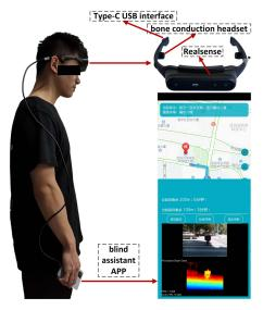
Fig. 2. The head-mounted assistive device for the blind (SensingAl G1): an RGB-D camera, a bone conduction headset, and a blind assistant app integrates the proposed system and GPS navigation.
