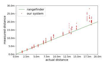
Fig. 12. The results measured by the rangefinder and the proposed system. x-axis: the actual distance; y-axis: the measured distance.
