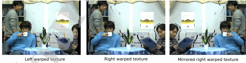
Figure 5: Occlusions in the left view appear to the right of objects, occlusions in the right view to the left. When the right view is flipped, occlusions appear on the right of objects, as for the left view ( Newspaper sequence).
