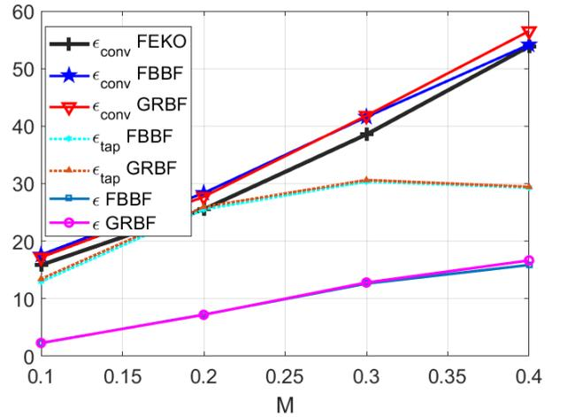
Fig. 2. Validation of the efficiency results for different modulation indices. The global efficiency  $\epsilon$  is the product between the aperture (tapering) efficiency  $\epsilon_{tap}$  and the conversion efficiency  $\epsilon_{conv}$ .
