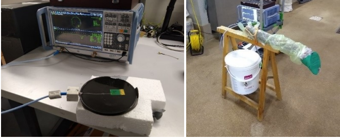
Fig. 4. The constructed pad (Left), the severed horse leg, covered in a hygienic veterinary glove. The part of the hoof is uncovered from the glove and the hoof pad is attached to it with tape. The cavity created between the hoof pad and the hoof is filled with Equi-pak. (Right)
