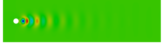
Figure B.8: POD (left) and calibrated ITSGM (right) pressure modes associated to the untrained Reynolds number Re = 195 .
