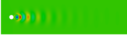
Figure B.8: POD (left) and calibrated ITSGM (right) pressure modes associated to the untrained Reynolds number Re = 195 .
