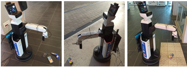
Fig. 5: The Toyota HSR performing precise positioning in different unknown environments.
