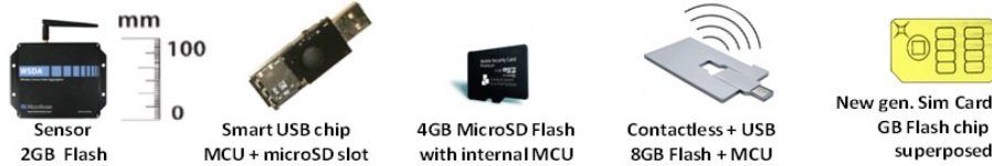
Fig. 2: Examples of cheap, low-end secure tokens that can be used in PAMPAS
