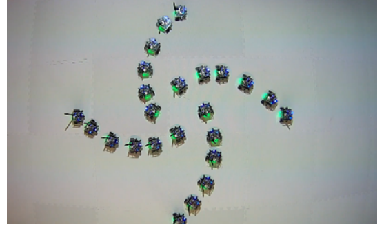
Fig. 6. Step 3: Experiments with Robotarium - Timelapse of robots' trajectories for the consensus example with N = 4 agents.
