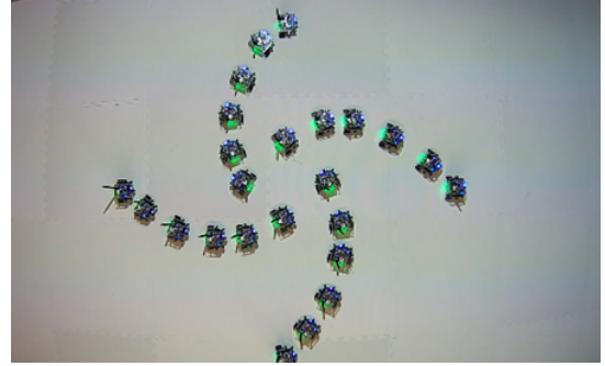
Fig. 6. Step 3: Experiments with Robotarium - Timelapse of robots' trajectories for the consensus example with N = 4 agents.
