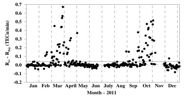
*Figure* 2.The variation R<sub>ev</sub>-R<sub>day</sub> at PHUT in 2011. R<sub>ev</sub>-R<sub>day</sub> values are presented by filled circles. The horizontal lines show 0.00 TECu/min and 0.04 TECu/min. The horizontal line at 0.04 TECu/min indicates the threshold for detection of ionospheric irregularity day
