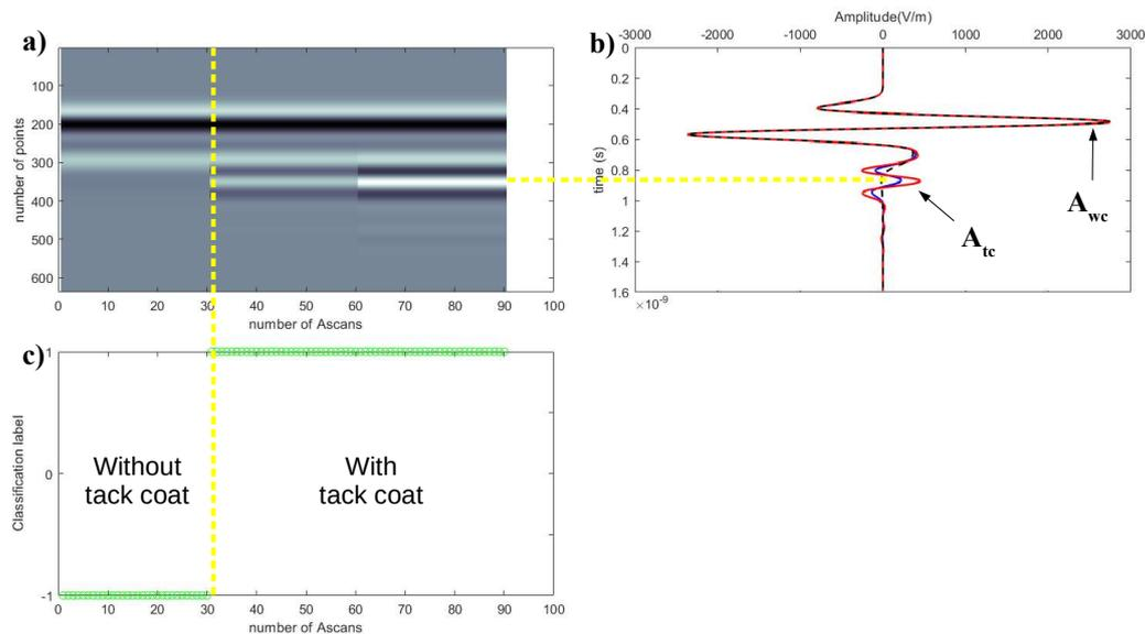
**Figure 3 a)** The B-scan (concatenation of A-scans, presented as examples) shows scanning of adhered and non adhered areas **b)** Time signals of the areas **c)** Classification of data using *Two-Class SVM* method, with and without tack coat
