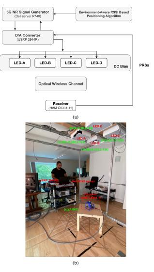
Fig. 7. (a)A flow chart of the demonstration, (b) Realistic scenario
