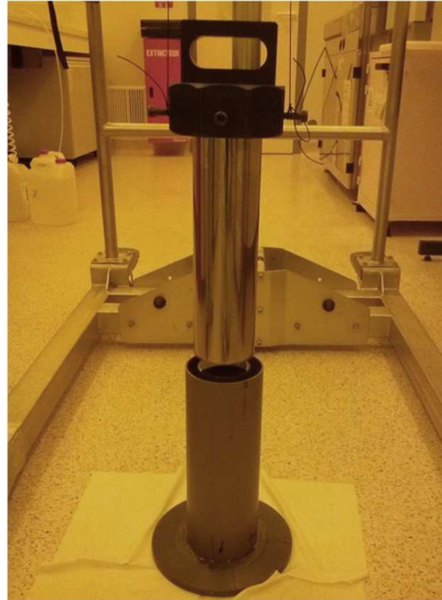
Fig.4. Dip coating pulley system used to deposit the photoresist on the tubular substrate.
