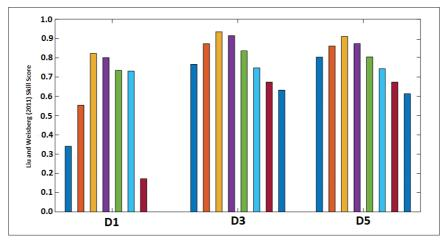
Fig. 1. Skill scores for the iSPHERE drifters (buoy deployments named here as D1, D3, D5). The wind drift-factor is varied between 0% and 7% at intervals of 1%.
