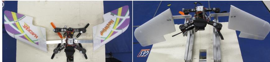
**Fig. 5** Examples of fixed configuration between the wing and the drone. Left figure is the system used in this paper for the experimentation that correspond to  $\alpha_D = 0$ , and right figure correspond to another configuration where  $\alpha_D = \pi/2$ .
