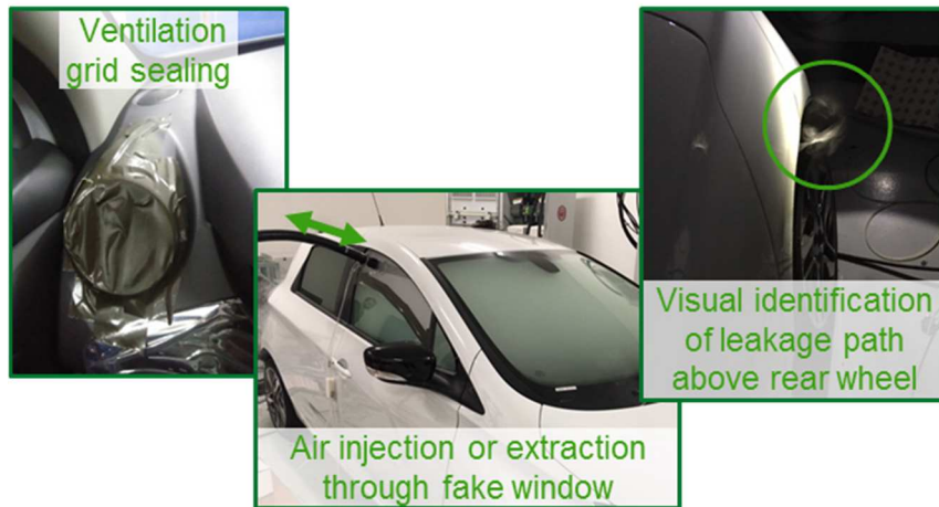
224 Figure 5 Test setup to identify leakage and infiltration paths of vehicle X.
