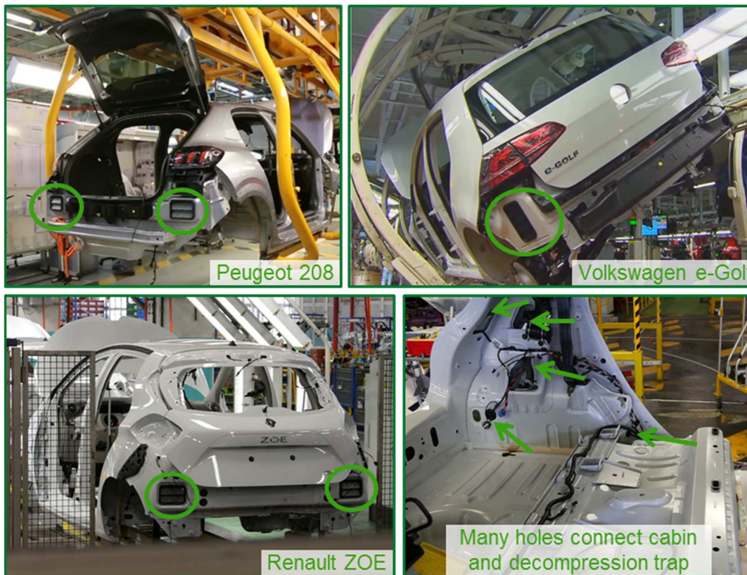
254 255 Figure 6 Decompression traps on various modern vehicles, and holes in the car body revealed during the 256 manufacturing process (PlaneteGT TV, 2019; Motor.TV, 2017; manufacturing, 2013)
