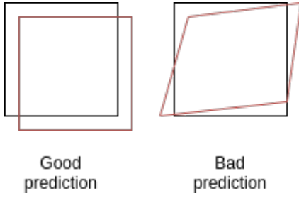
FIGURE 4 Example of two predictions (red) that have similar errors compared with the ground truth (black). The right-hand side prediction is 22% more accurate than the left one according to the MSE, yet we would prefer the left one that better preserve some physical properties.
