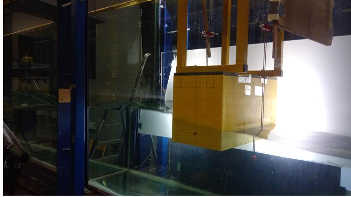
Figure 18: Photograph of the experimental set-up of the rectangular barge in the wave flume (the wave maker is on the left side).
