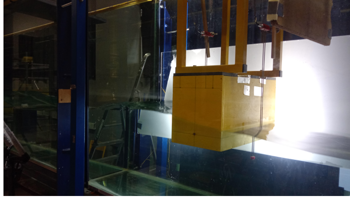
Figure 18: Photograph of the experimental set-up of the rectangular barge in the wave flume (the wave maker is on the left side).
