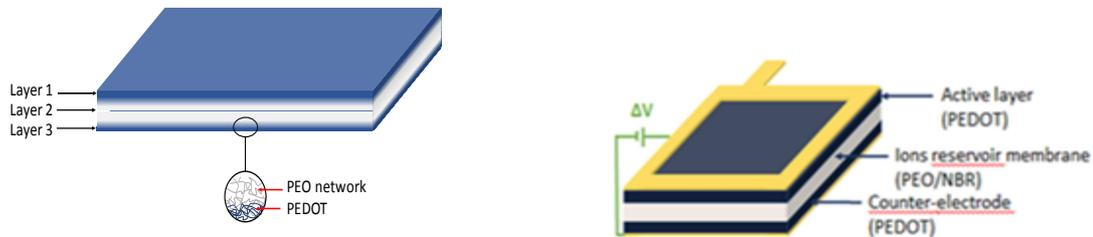
Figure 4 : Schematic representation of the tri-layer NBR/PEO/PEDOT IPN (up) and its connexion frame (down)
