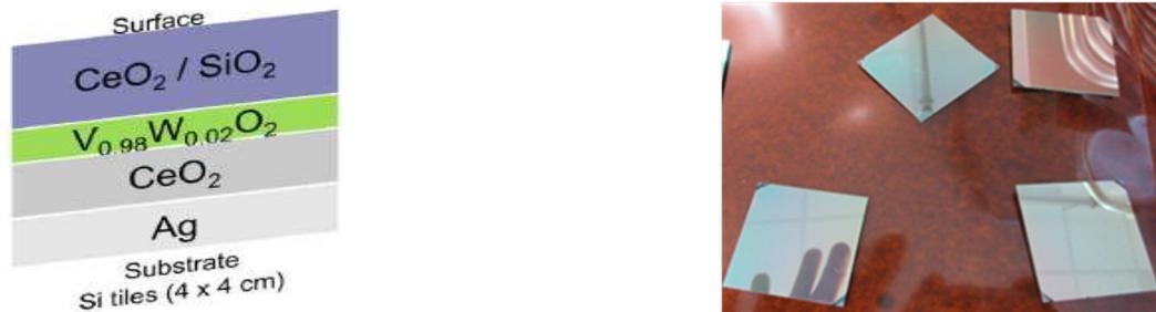
**Figure 2 : TCH multilayer stacking (patented design<sup>5</sup>) (left), 40x40mm<sup>2</sup> solar protected TCH tiles (right)**
