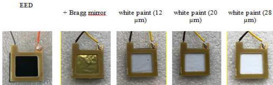
**Figure 6 : Images of single EED connected and covered with various coatings**
