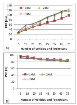
Fig. 8. RTD and PDR vs. Number of Vehicles and Pedestrians (LTE Connection with the Fog Node)
