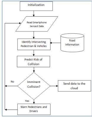
Fig.2. Flowchart of Pedestrian Collision Prediction Algorithm
