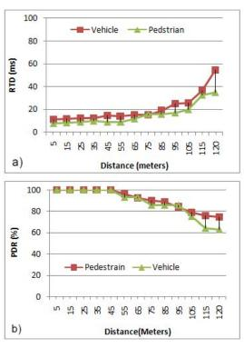
Fig. 5. RTD and PDR vs. Distance (WiFi connection with the Fog Node)
