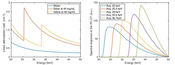
Fig. 1. Left: lines of the  $\Sigma$  matrix corresponding to the linear attenuation coefficient of iodine in solution at 40 mg/mL, silver in solution at 40 mg/mL and water. Right: Normalized columns of the  $F$  matrix corresponding to the 5 spectral responses of the 5 simulated tomographic acquisitions.
