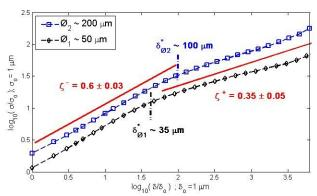
Figure 4: Effect of disorder on the self-affine scaling of interfacial crack fronts. We plot the standard deviation  $\sigma$  of the height fluctuations  $\Delta h(\delta)$  of the crack interfaces as a function of the scale  $\delta$ . We analyzed two different sets of data, prepared with glass beads of different diameters respectively  $\emptyset_1\sim 50 \mu m$  and  $\emptyset_1\sim 200 \mu m$ .
