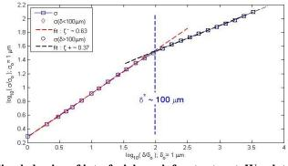
Figure 2 : Scaling behavior of interfacial crack fronts at rest. We plot the standard deviation  $\sigma$  of the height fluctuations  $\Delta h(\delta)$  of the crack interfaces as a function of the scale  $\delta.$  The glass beads used for preparing the samples – blasting and roughening of the Plexiglas plates – had a diameter of  $\varnothing_2 \sim 200~\mu m.$
