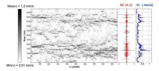
Figure 3: (a) Spatio-temporal of the local velocity of the crack front during its propagation within the weak heterogeneous plane of the Plexiglas block at an average speed of  $\langle V \rangle \approx 200~\mu m/s$ . (b) Acoustic emissions continuously recorded by one contact microphone, output signal in volts (Arbitrary Units) (Wide Band acoustic sensor 100kHz - 1MHz) at 1MHz during the crack propagation. (c) The average crack front speed shows an intermittent dynamics.
