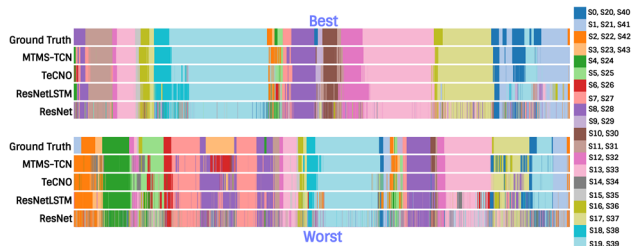
Fig. 7 Step recognition on complete videos in Bypass40 for quality assessment. The figure shows best (top) and worst (bottom) performance of our model. The 44 distinct steps are mapped to the same 20 categorical colormap
