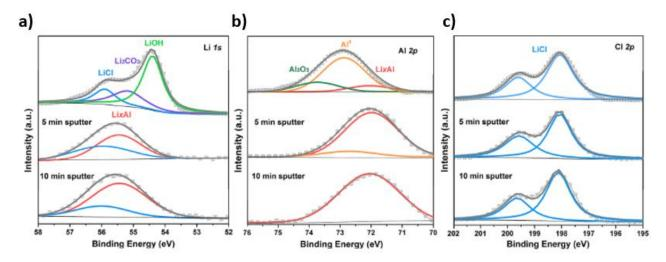
Figure 2. XPS analysis of the lithium electrode treated with AICl<sub>3</sub>-THF solution before and after Ar sputtering: (a) Li 1s, (b) Al 2p and (c) Cl 2p spectra. Analysis performed after argon sputtering suggests a uniform distribution of LiCl in the whole coating layer. Reproduced with permission from Ref. [49]. Copyright 2020, Elsevier
