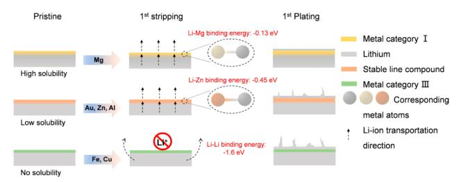
Figure 6. Protective mechanisms for Li plating/stripping depending on the nature of the metals solubility.
