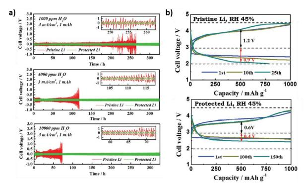
Figure 9: Electrochemical behavior of lithium electrode in humid atmosphere during in symmetric cells (a) or in  $Li/O_2$  cells (b). In both cases, electrodes protected by a preliminary treatment with  $GeCl_4/THF$  steam exhibit better stability and lifetime, and less polarization. Adapted with permission from Ref. [65], Copyright, 2018, Wiley.
