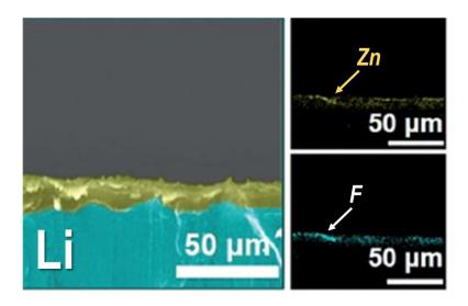
Figure 1. Example of cross-section SEM images for charactering the coating. Here, lithium electrode is protected by immersion in  $ZnF_2/(DOL:DME)$  dispersion. The EDX mapping on the right confirm the deposition of zinc, as well as the presence of fluorine in the by-product LiF. Adapted with permission from Ref. [50], Copyright 2019 Royal Society of Chemistry.
