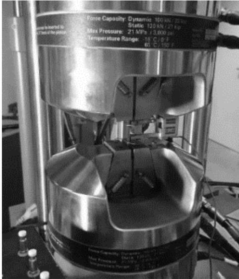
Fig. 5 –Tensile test machine including extensometer.
