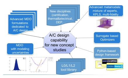
Fig. 4. MDAO framework for A/C design [43]
