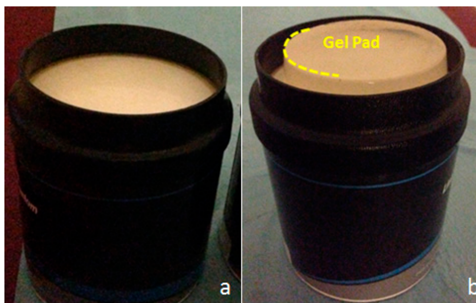
Figure 2. Phantom model 039 “Shear Wave Liver Fibrosis Phantom” (CIRS, Norfolk, VA). (a) One example from the series of four homogeneous phantoms of different stiffness (3.5, 11.4, 28.6, and 44 kPa). (b) Modified depth: 2 cm gel pad added to measure at 9 cm depth avoiding “edge effects”.
