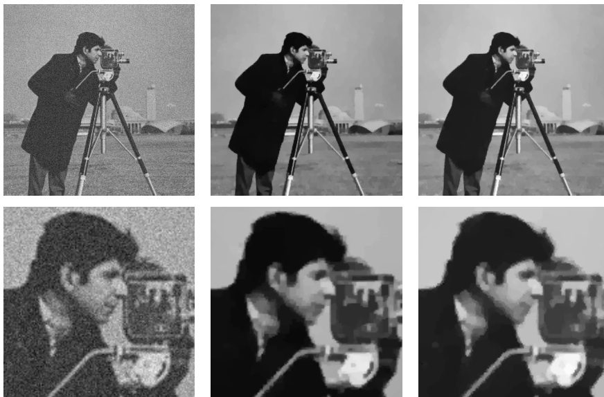
FIGURE 9. “ROF” denoising example. Left: noisy image. Middle, denoised with \varphi(\nu) = |\nu_1| + |\nu_2| . Right: with the effective tension computed for T = 4 .
