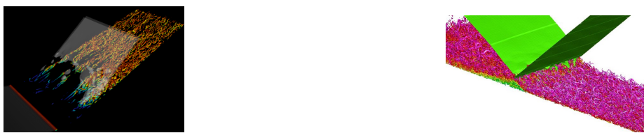
Figure 1: Q criterion colored by the magnitude of the longitudinal velocity. Shock waves are highlighted by isosurfaces of \nabla \cdot \mathbf{u} : laminar case on the left, turbulent case on the right.
