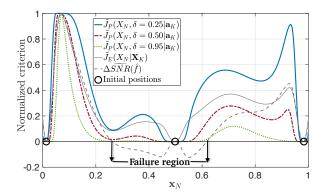
Fig. 5: Effect of parameter  $\delta$ . The solid curves are the proposed criterion for different  $\delta$ . The superscript tilde represents the normalization of the function. By increasing  $\delta$ , the algorithm is more robust against FR. However, other candidates for sensor placement which provide significant increase in the SNR can be ignored.
