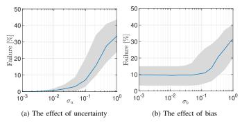
Fig. 3: Failure [%] is a measure to compute the ratio of the sensor placement region which is in the failure region. (a) In this figure, the effect of the uncertainty level on the Failure [%] is depicted. Here, the bias is considered to be equal to 0. (b) The effect of bias on Failure [%] is depicted in this figure. The variance of the uncertainty is set equal to  $\sigma_u = 0.01$ .
