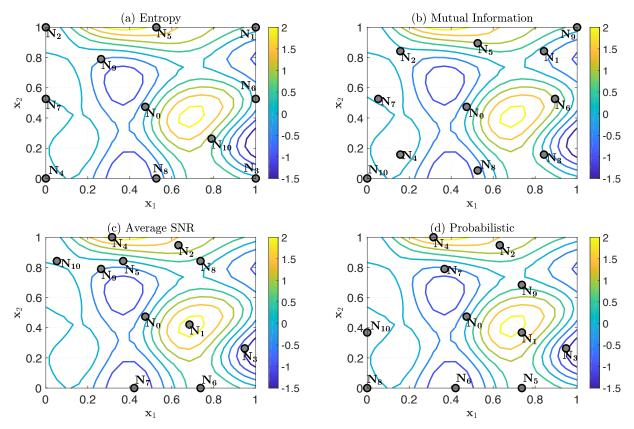
Fig. 9: This figure depicts the sensors' positions obtained from different criteria in a 2D space, by choosing one realizations of the spatial gain and the noise. The contour represents the true values of the spatial gain. We note that based on Fig. 8 the final output SNR for 100 MC realizations is reported 11, 14, 16, and 23 (in dB) respectively for  $J_{MI}$ ,  $J_{H}$ ,  $J_{E}$ , and  $J_{P}$ .
