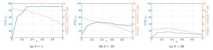
Fig. 6: The trade-off between the robustness and the maximization of the averaged SNR improvement can be controlled by changing the parameter  $\delta$ . The blue curve with y-axis on the left represents the average FPR[%] according to different levels of uncertainty, and the orange curve with y-axis on the right depicts the average improvement of the SNR. From left to right, figures (a), (b), and (c) show the results for different values of  $\delta$ .
