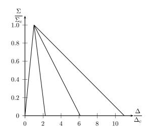
Figure 9: The sharp interface for a cavity :  $\sigma_{rr}(R)$ , for  $R/R_e = .2, .4, 1, R_i/R_e = .1$
