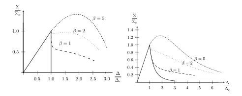
Figure 1: Homogeneous response of the bar, left :  $\alpha = 0$ ,  $h_o = 0$  and  $h_o = 10, \beta = 1(-), 2(.), 5(--)$  right:  $\alpha = 1$ ,  $h_o = 0$  and  $h_o = 10, \beta = 1(-), 2(.), 5(--)$ .
