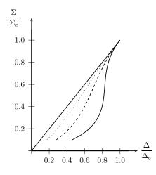
Figure 5: The bar in extension :  $\omega = 1 - d, h = 0$ , depending on L :  $L = l_c, " - "; L = 2l_c, " - ", L = 3l_c, "."$
