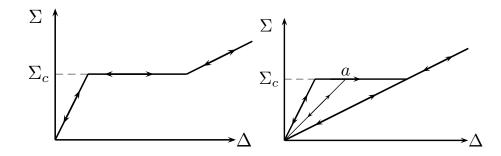
Figure 3: Reversible Phase transformation, (Left) ; with dissipation (Right) ; <-> reversible path
