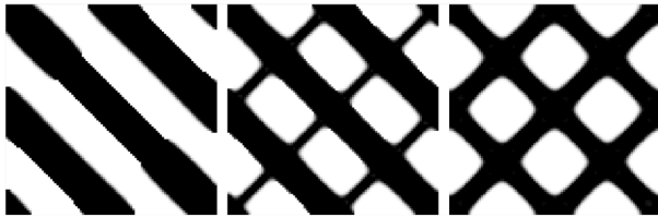
(c) Micro-structures obtained for different cubicity values : 0, 0.5 and 1
