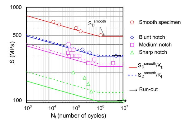
Figure 11: Life predictions versus S-N data for the base metal
