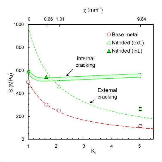
Figure 12: Fatigue strength at 10<sup>6</sup> cycles versus stress concentration factor K<sub>t</sub> and relative stress gradient  $\chi$
