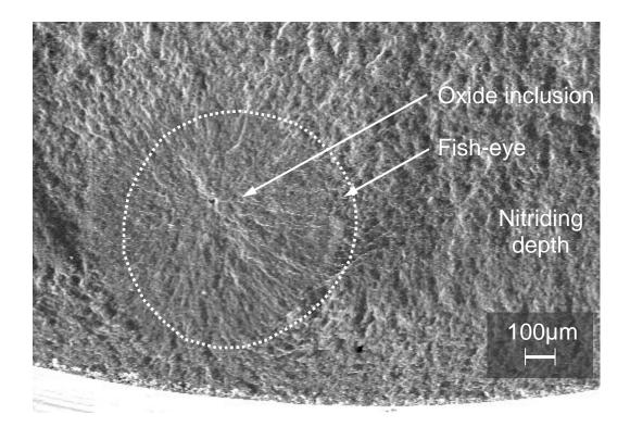
Figure 8: Fish-eye crack nucleated under the diffusion layer at a nitrided blunt notch (575MPa, 389,216 cycles)
