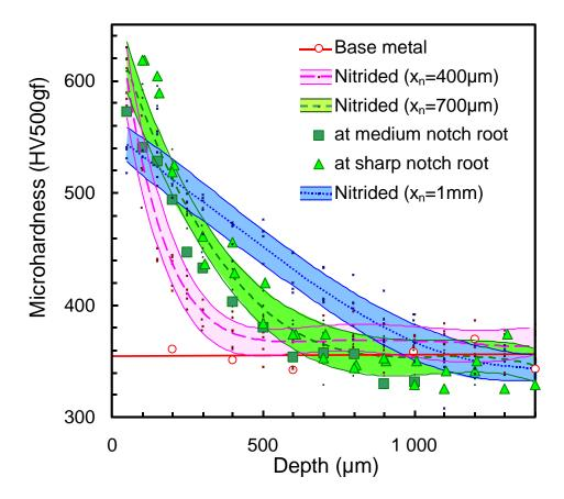
Figure 4: Microhardness profiles with scatter-bands for the three nitriding depths in smooth specimens and microhardness data at medium and sharp notch roots for  $x_n = 700 \mu m$
