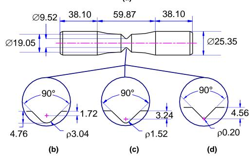
Figure 1: Dimensions in mm of smooth and notched cylindrical specimens used for fatigue testing
