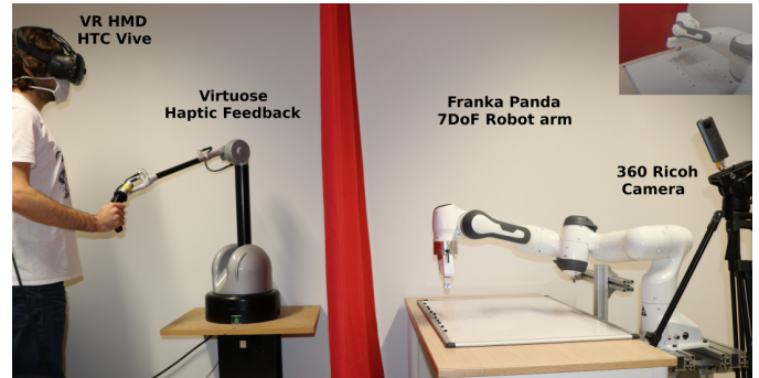
Fig. 1. Embodied teleoperation setup. Our setup consists of a Virtuose haptic device and a Franka Panda robot. The operator wears a head mounted display and operates the robot using the haptic device. He is provided with a first person visual display from a camera placed above the Franka. The controller utilized to help him guide the trajectory and impedance of the robot is explained in Sect. II. The setup can be seen in use in the demonstration video 2
