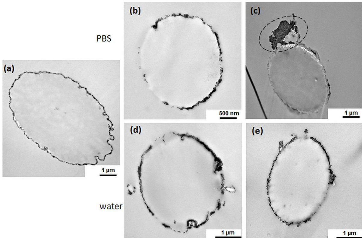
**Figure 2. *In vitro* degradation of PLA@SPIONs.** TEM images of PLA@SPIONs nanofibers before (a) and after degradation in PBS solution (37°C, pH 7.4) 1 week (b) and 1 month (c) or in water (37°C) (d) 1 week and (e) 1 month.
