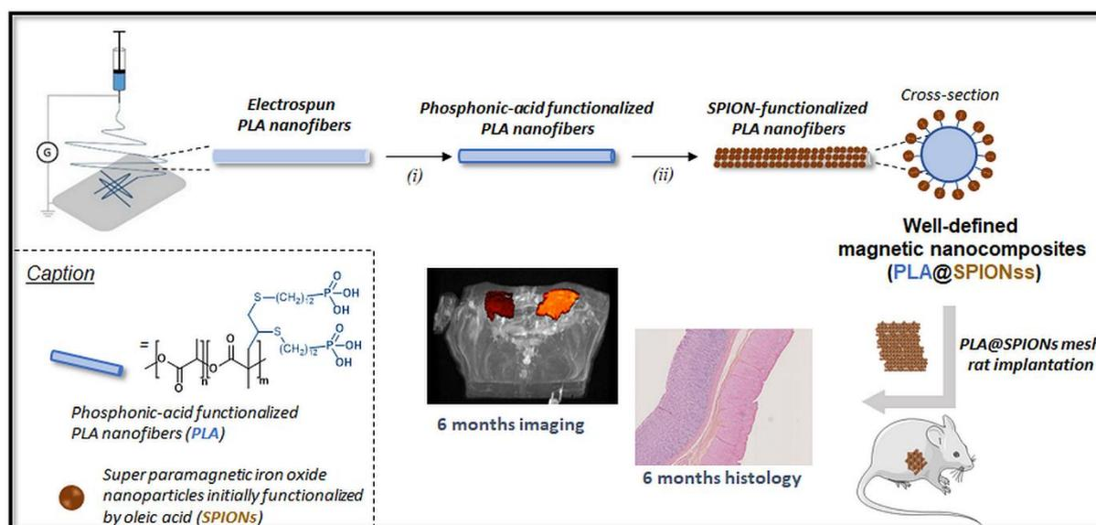
**Scheme 1.** Schematic representation of the synthetic strategy followed for the preparation of well-defined magnetic nanocomposites PLA@SPIONs and overview of the *in vivo* studies performed. i) functionalization of the PLA nanofibers surface with phosphonic acid groups and ii) ligand exchange procedure to anchor SPIONs at the surface of the phosphonic-acid functionalized PLA fibers.
