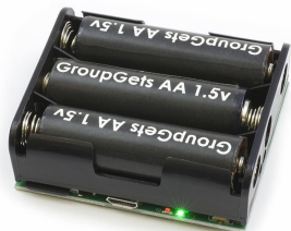
Figure 4: Left: Printed circuit board (PCB) of the AudioMoth sensor. Right: battery holder. Photographs reproduced from the official website of Open Acoustic Devices.
