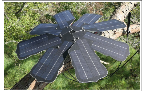
Figure 5: The RFCx Guardian acoustic sensor, equipped with eight solar panels and deployed in a tree. Photograph credit: Aya Naboulsi, Rainforest Connection.
