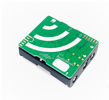
Figure 4: Left: Printed circuit board (PCB) of the AudioMoth sensor. Right: battery holder. Photographs reproduced from the official website of Open Acoustic Devices.
