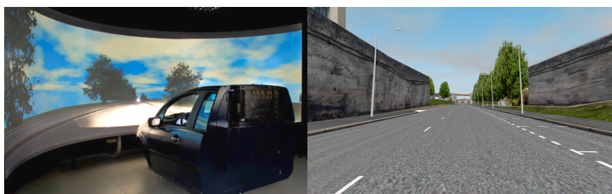
Fig. 4. Picture of the driving simulator and the driving scene used for the perceptual study.
